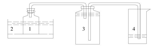
**Figure 1:** Sketch of lab-scale digester and biogas collection apparatus used in the laboratory experiment (1—11 Glass flask (Digester), 2—Thermostat water bath, 3—21 Glass container (collecting biogas), 4—Measuring cylinder)
