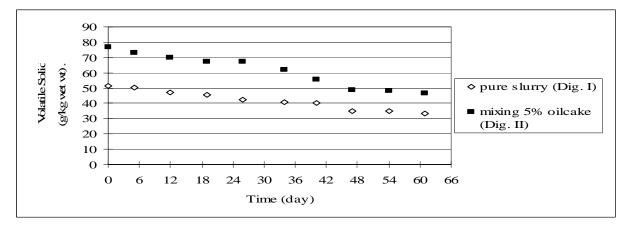
Figure 4: Variation of volatile solid in both digesters
