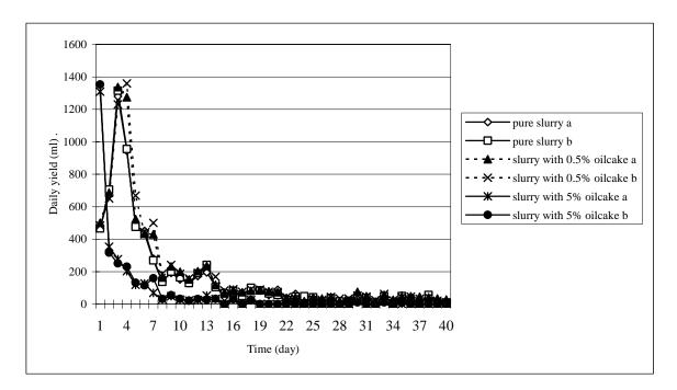
Figure 10: Daily biogas production for lab-scale fermentation
