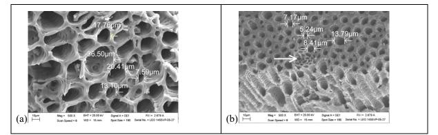
Figure 1. Morphology and pore sizes of CB from (a) 400 °C-6h and (b) 600 °C-4h
