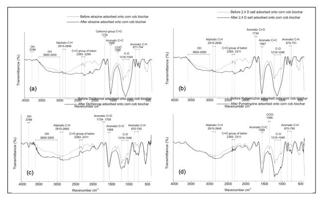
Figure 2. FTIR of corn cob biochar for both before and after adsorbed pesticides (a) atrazine, (b) 2,4-D, (c) dichlorvos, and (d) pymetorzine.
